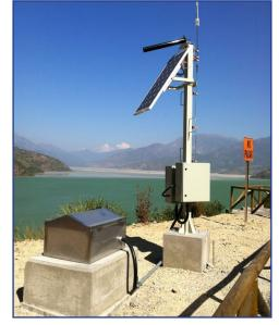
Solar panels were also set up with large-capacity batteries to power the GSR-18 units with AC-63 accelerometers synchronised with GMS timing.
